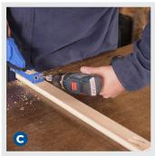
C Rotate Reel Support Brace and drill two pocket holes in the opposite end.
