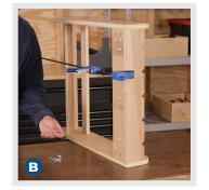
Align Top Brace into assembly so it is flush with the back of the end pieces and snug against the Fishing Rod Holder.
