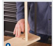
A Clamp Bottom Board to one Side Board using the reference lines to align the pieces at the correct angle.
