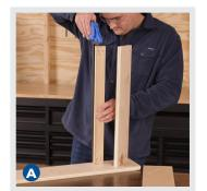
A Clamp Reel Support Brace to Side Board using reference lines to align pieces
