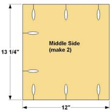
**Step 11:** Cut two Middle Sides to size from 3/4" plywood. Also cut two Middle Stiles from 1x2 boards. Then, with your Kreg Jig® and bit reset for 3/4" material, drill pocket holes where shown. Once again, these parts are symmetrical, so they can be used on either side.
