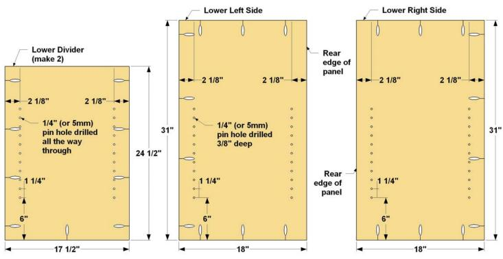
Step 5: Cut a Lower Left Side, Lower Right Side, two Lower Dividers, and four Lower Shelves to size from 3/4" plywood, as shown in the cutting diagram. Next, use your Shelf Pin Jig to drill holes for shelf pins. Note that in the Sides, the holes are 3/8" deep—the standard drilling depth for the Shelf Pin Jig. On the Lower Dividers, the holes go all the way through. You'll actually drill in from each face using the jig, but that will effectively create holes that go all the way through.
