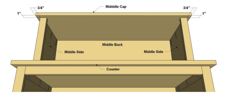
**Step 13:** Cut a Middle Cap to size from 3/4" plywood. While you're at it, cut the Top Cap, as well. They're the same size. If desired, apply edge banding to the front and side edges. Now attach the Middle Cap to the middle structure. You'll use 1 1/4" Kreg Screws in the Sides, and 1" Kreg Screws in the Back.
