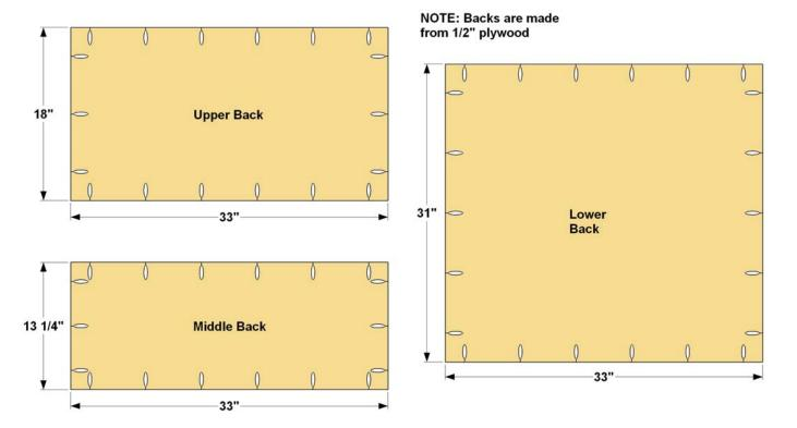
Step 9: Cut a Lower back to size from 1/2" plywood, as shown in the cutting diagram. While you're at it, you can go ahead and cut the Middle Back and Upper Back, as well. They're all the same width. Only their heights differ. Set your Kreg Jig® and bit for 1/2" material, and then drill pocket holes in the Backs, as shown.
