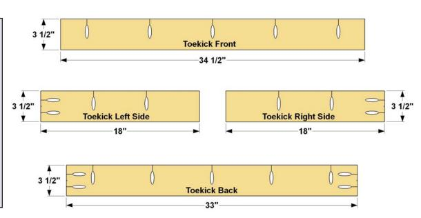
Step 3: Assemble the toekick structure using 1 1/4" Kreg Screws. NOTE: If you're building from a softwood, such as pine, choose coarse-thread screws. If you're using a hardwood, choose fine-thread screws instead.
