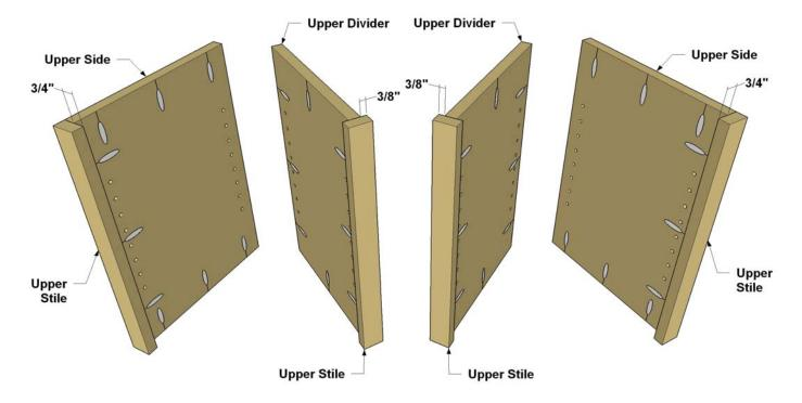
**Step 15:** Cut four Upper Stiles to length from 1x2 boards, and then attach them to the Upper Sides and Upper Dividers, as shown. Again, this is similar to creating the Lower Sides and Lower Dividers.
