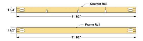
Step 7: Cut a Frame Rail and a Counter Rail to length from 1x2 boards, as shown in the cutting diagram. Also cut two Slide Spacers to length from a 1x4. Then drill pocket holes in the Rails where shown. Note that the Counter Rail has holes along the upper edge for attaching it to the Counter.
